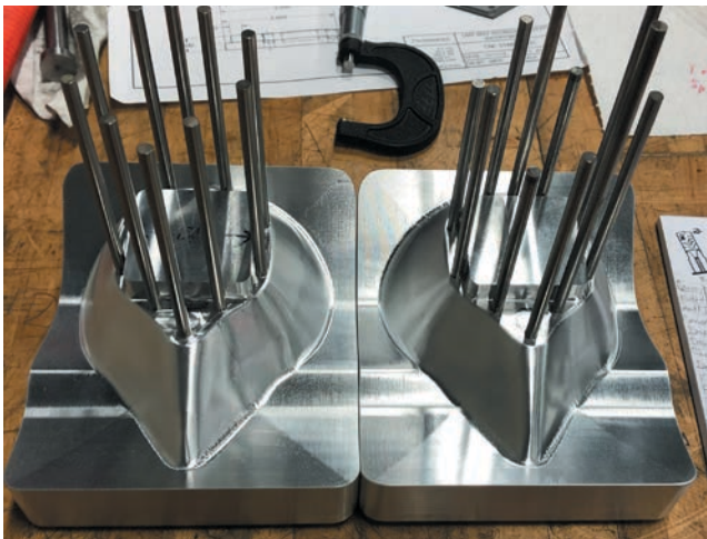
Illinois-based manufacturer, Progressive Components, donated mold components for LATI projects, including the ejector pins for the mold, shown here in a test fitting for the cores.
