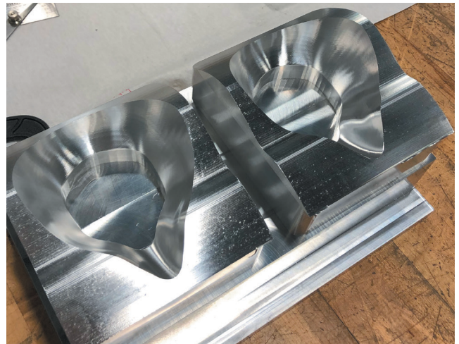
Cavities and cores were machined on a Mazak Nexus 410 machining center, using CNC programs generated with GibbsCAM.
