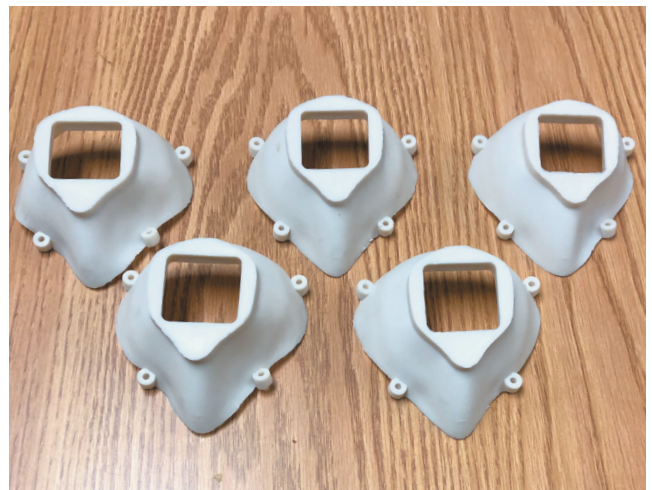
After testing the mold by making these prototypes, the team adjusted the mold, obtained a more flexible thermoplastic rubber, and began production, molding a pair of mask shells every 80 seconds.
